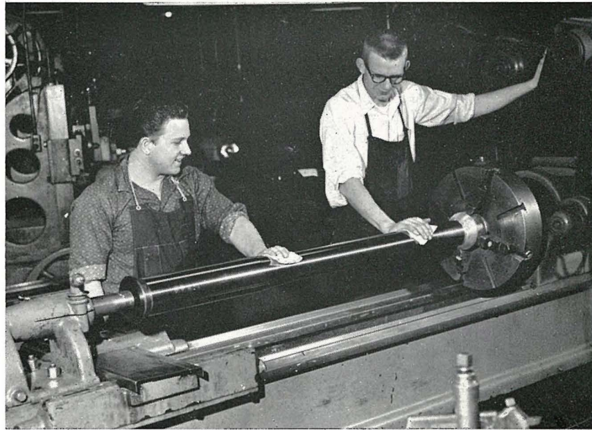
Vocational students, James Coleman and Jerry Daniels, polish a piece of cold roll steel to be used by an industrial plant in southern Ohio.
